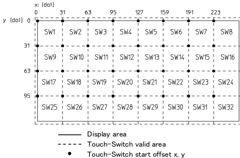
\* Touch-Switch start position may be offset by a number of dots, so an appropriate margin should be incorporated into the display pattern when using adjacent switches.
