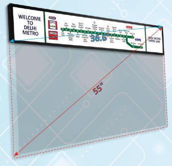
Resizing LCD technology transforms a standard LCD into a **custom ultra-wide format** by precisely cutting the glass, circuits, and polarizers — without sacrificing performance. This innovation allows **unique aspect ratios** for modern signage, transportation, kiosks, and industrial applications.
